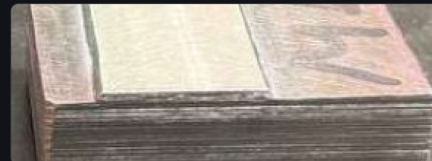
Machined sample — hardfaced valve disc after surface preparation
